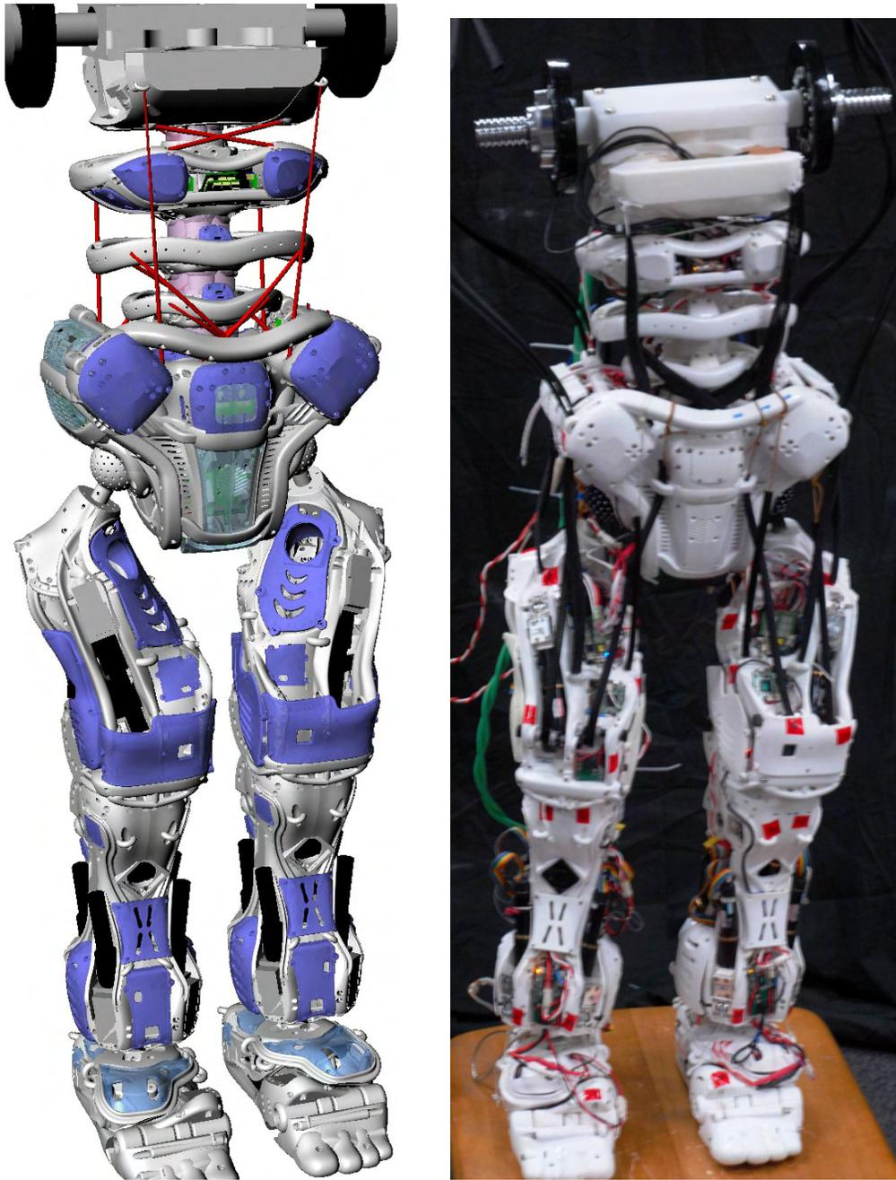
Fig. 4. Current status of Kojiro (left: CAD, right:real photo)
