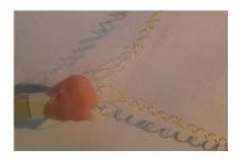
The next step is to manufacture and attach the cone. The glass cone is shaped by heating and pulling a thin walled borosilicate microfilament glass rod of wall thickness 0.125mm and diamter 1 mm (AM Systems Inc). The electrode puller (Kopf model 720) has settings of 12.5 for the heater and 1.0 for the solenoid that applies the pull. The lower
