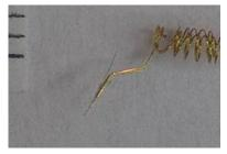
end is shaped by breaking the tip with forceps until the tip diameter is 50 to 100 microns. The upper end is shaped by using a diamond knife to cut the glass. Prior to cutting, a piece of fine wire (one strand of a stainless steel wire) or fine hair is inserted into the lower end so that when it is cut off and moves away, it can be easily retrieved and held with fine forceps. The upper end is broken back with forceps until it measures about 300 -
