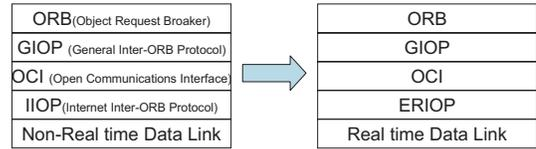
Fig. 10. Difference between conventional and real-time CORBA
