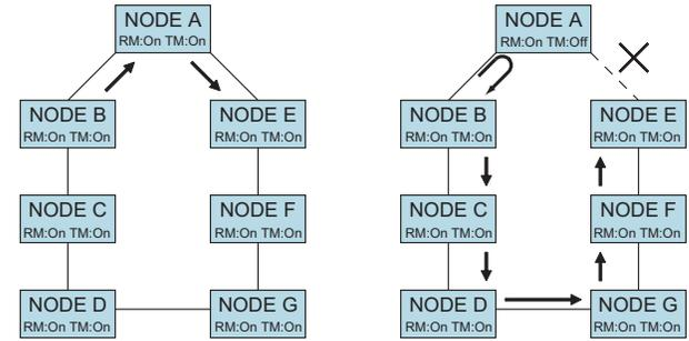
Fig. 4. Route reconfiguration(RM:Relay Mode, TM:Through Mode)
