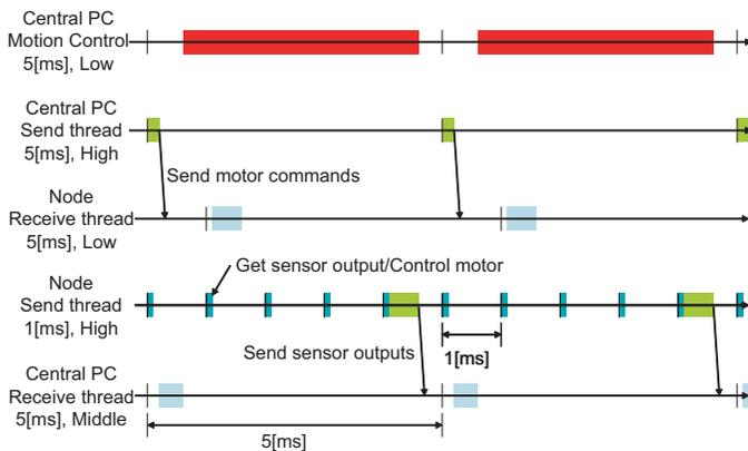
Fig. 13. Time chart of distributed I/O software
