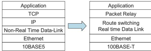
Fig. 3. Difference between conventional and real-time ethernet
