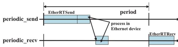
Fig. 7. Time chart of real-time communication program
