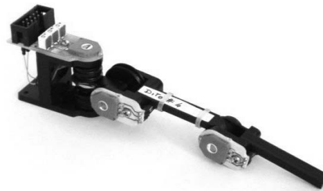
Fig. 2. Skeleton of the fingers with joint sensors.
