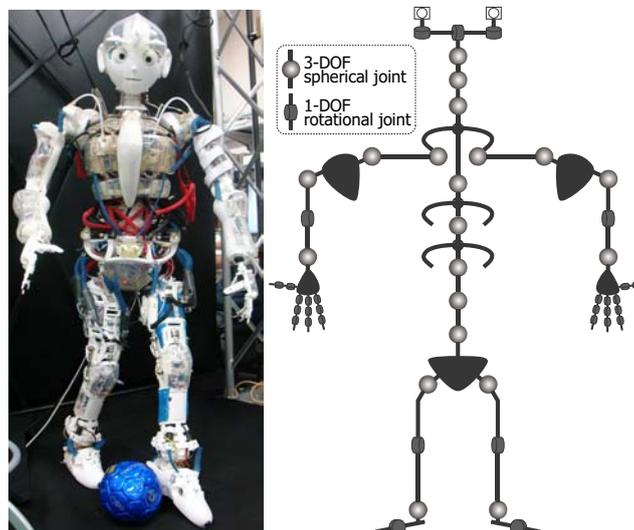
Fig. 1. Kotaro's photograph (left) and the arrangement of joints (right).
