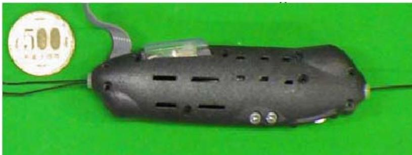
Fig. 2. A newly-developed, sensors-integrated muscle unit.
