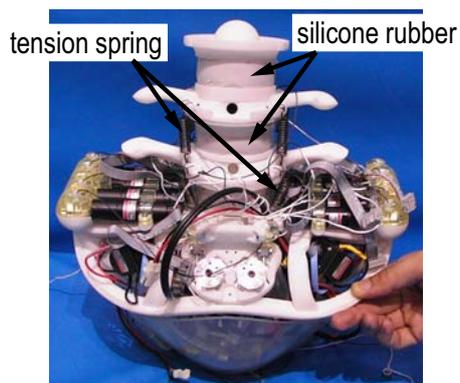
Fig. 6. Elastic and viscous elements between joints.
