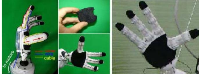
Fig. 11. Soft and fleshy tactile sensor using conductive rubber foam.
