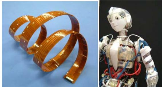
Fig. 12. Free form tactile sensor for covering whole body.
