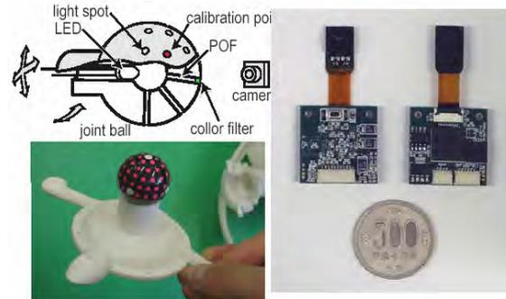
Fig. 13. Posture sensor for ball-and-socket joint using a mobile phone camera and a mobile phone microprocessor.
