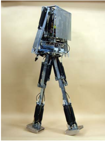
Figure 1: An anthropomorphic biped walker “Pneumat-BT”. It has 13 degrees of freedom and 26 McKibben artificial muscles.
