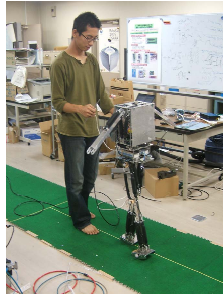
Figure 7: Experimental setup: the anthropomorphic biped robot “Pneumat-BT” walks on a flat carpet.
