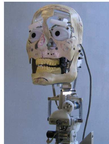
Fig. 1. The humanoid robot head "ROMAN" (ROMAN = ROBot huMan interAction machiNe) of the University of Kaiserslautern.
