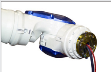
THRU-ARM CABLE AND HOSE ROUTING
