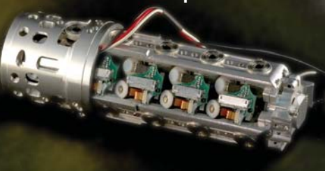
Here are the stackable pucks (right end) and the motor assembled for the 15-dof prosthetic hand.
